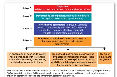
Figure 2: Four-level model for the specification of performance of buildings and construction works
